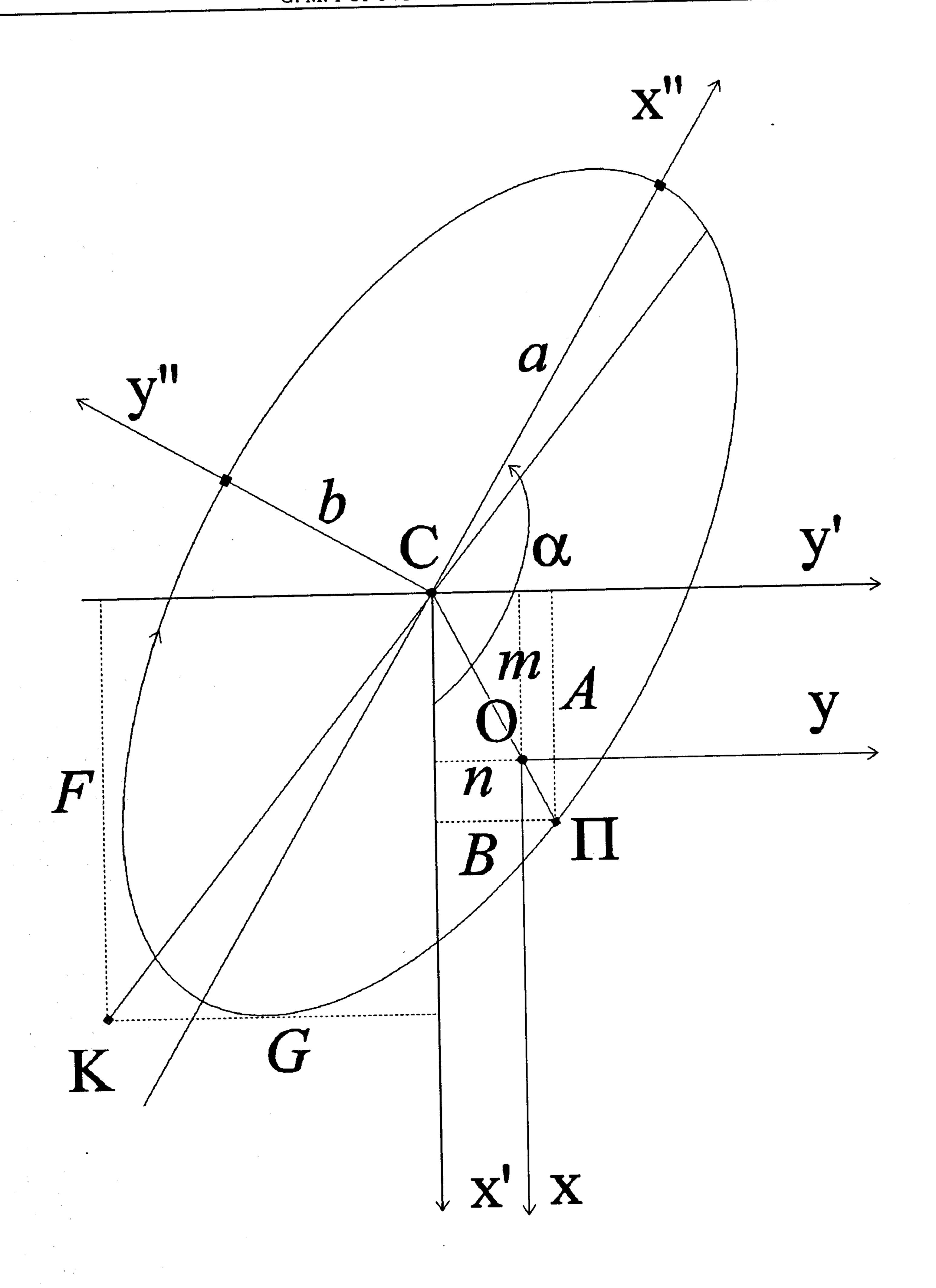
Figure 1. Geometrical meaning of the Thiele-Innes elements.
